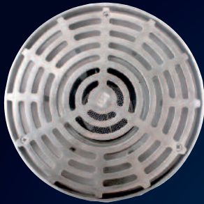
SPS 225mm round push-in floor drain. 316 stainless steel with 150mm outlet.
