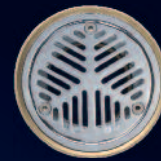
Vinyl floor waste. Chrome on brass or 316 stainless steel grate with o-ring seal into 80mm or 100mm diameter pipe.
